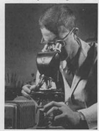
BASIC TOOL of the Microchemistry Laboratory is the microscope. Here Lew Jones studies a plastic replica specimen from a contact to optically analyze foreign matter on its surfaces. Area under observation is somewhat smaller than this period.
